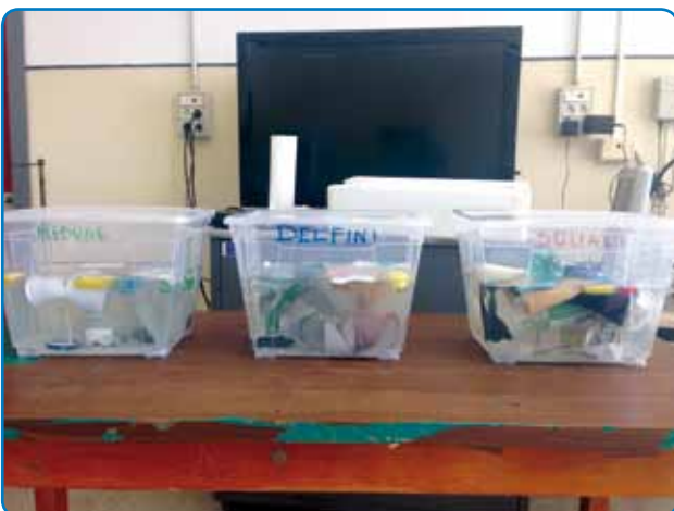
Figure 86. Experiment setting for testing degradation times of several macrocategories of litter
